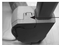
Step 1: Insert e.g. a screwdriver at a 45 °C angle as illustrated.
