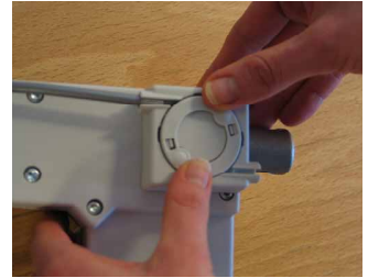
Fig. 3. Replacement of QR cover.
