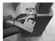
Step 2: Turn the screwdriver to release the cable lock.
