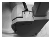
Step 1: Insert e.g. a screwdriver at a 45 °C angle as illustrated.
