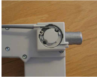
Fig. 2. QR cover removed.
