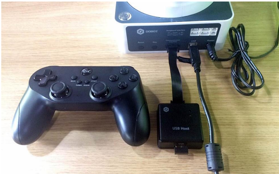
Figure 12.5 Installation of Beitong Joystick
