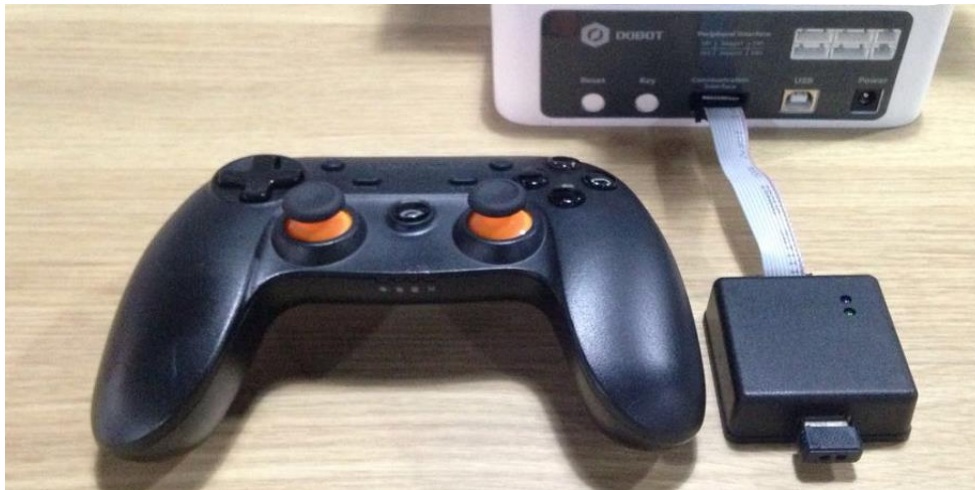
Figure 12.1 Installation of stick module
